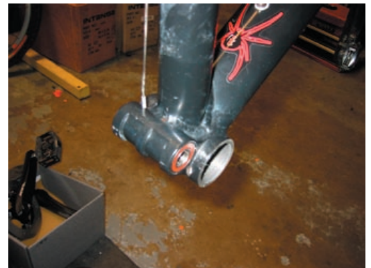
(picture of installed bearings in bottom bracket pivot)
