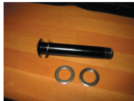
(picture of pivot bolt with spacer, grease and loctite)
