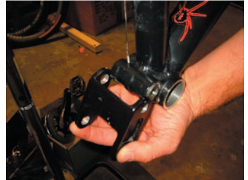
(picture of bottom bracket pivot with spacers held on by grease, and box link ready to go on)
