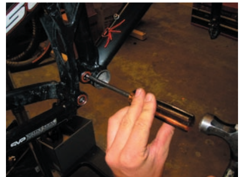
(picture of screwdriver inserted through bearing)
