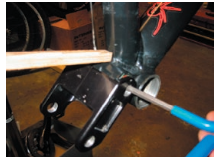
(picture of allen wrench through box link to locate spacers)
