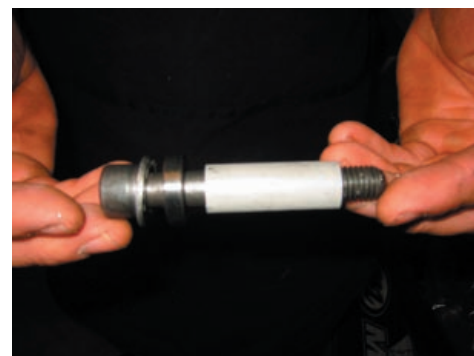
(picture of assembled bearing press, bolt, washer, bearing, & crush tube)
