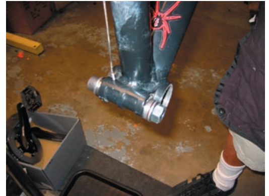
(picture of press assembled and finger tight on bottom bracket)
